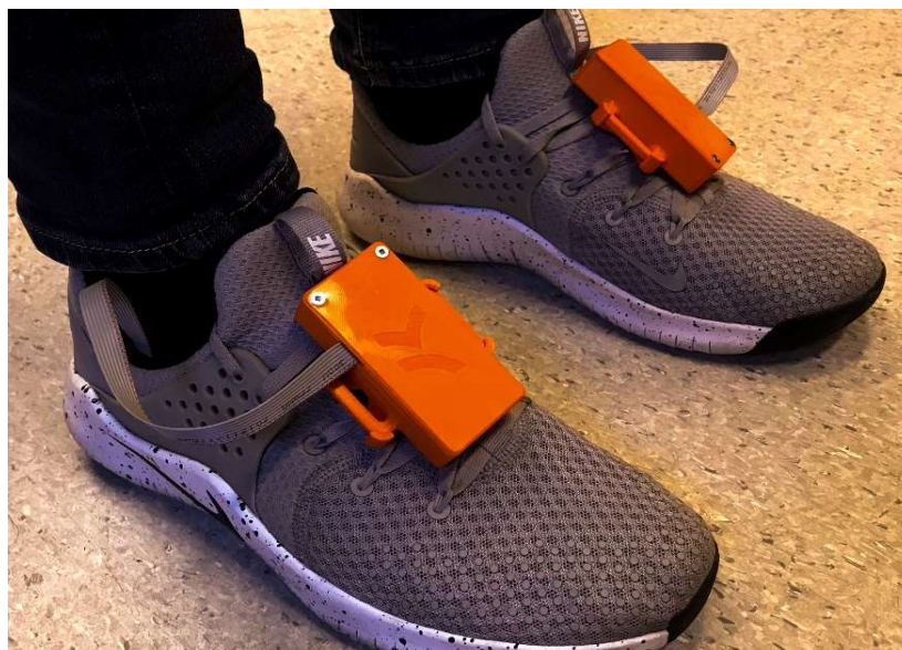
Figure 1 - Participant wearing the Posture differentiating Insole (PDI) system
